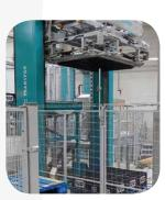
The layers are prepared prior to entering the palletiser using dividers and turners Capacity: 400 layers per hour on depalletisation, 360 layers per hour on palletisation
