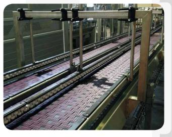
A conveyor of proven resistance capable of supporting heavy product flow (boxes, packs, racks...)
